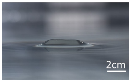
Figure 1: Image of a deformation of the water-air interface by combining two ultrasonic transducers.
